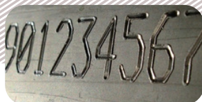
Deep marking on steel
